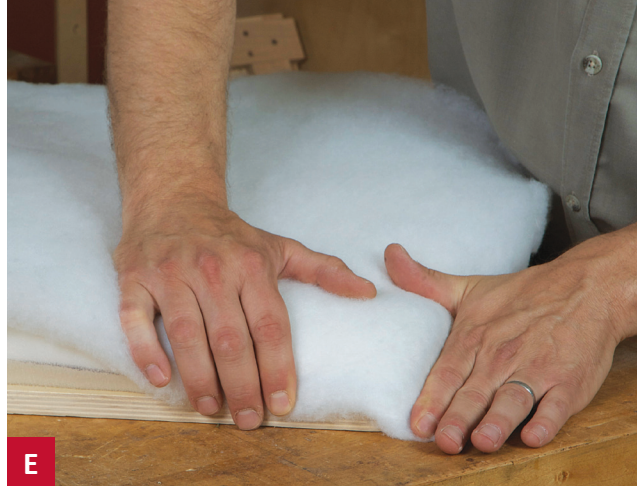
E Fit the polyester fiber onto the foam. Trim back any extra that runs over the edge of the plywood.
