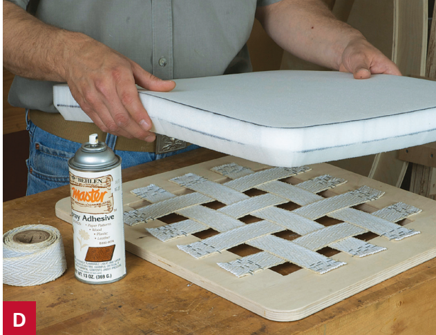
D Align foam with plywood carefully. Spray on adhesive and apply downward pressure to ensure good bond.
